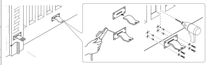
Insert the bushing (lubricated) into the pillar bracket's hole. The bracket has holes that allow the opening angle to be changed. Secure the tail joint to the bracket. Secure the tail joint to the bracket.
