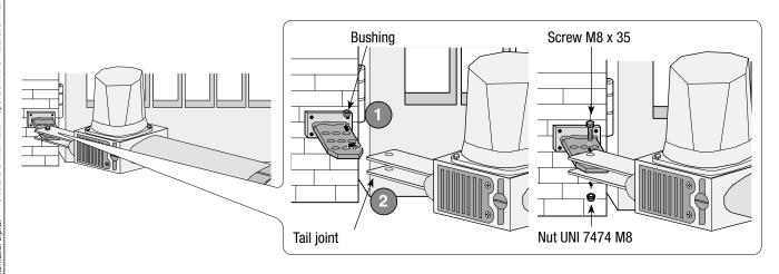
Insert the bushing onto the main lug as shown in the drawing.
