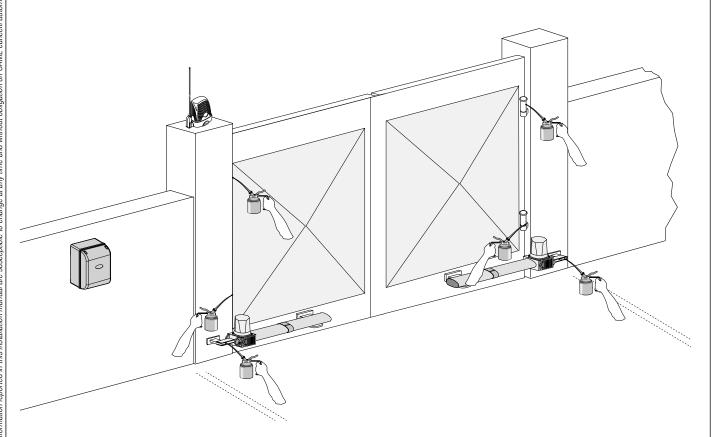
Make sure there are no plants within the photocell's beam, and that the gate motion is free of any obstacles.
