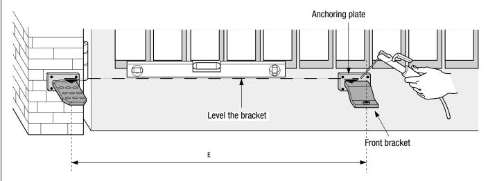
Assemble and weld the two parts of the pillar bracket. Secure the bracket to the point you have chosen with proper plugs and screws or - if the pillar is made of metal - weld it on.
