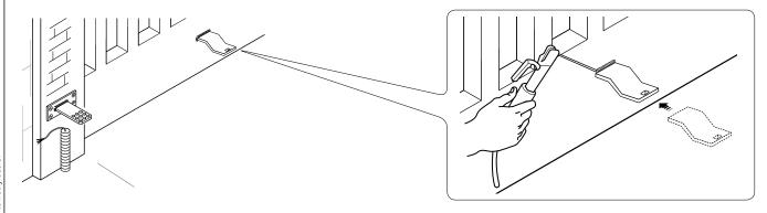
Note: on non-metal gate leaves assemble and weld the two parts of the bracket and secure them with proper screws.
