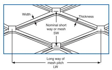
2) For **FLATTENED MESHES** dimensions of the aperture point to point are shown.
